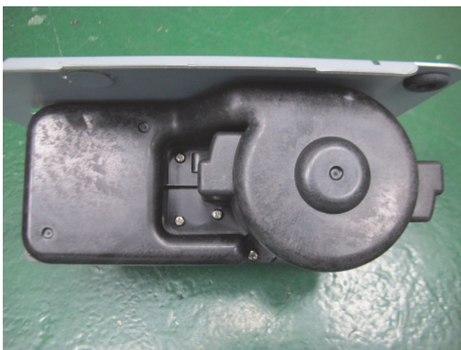
2. Loosen the fixing screws of the blower and remove the blower housing.
