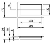
Punched fixing holes Ø5 in sides
