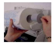
To load the first roll plug the plastic holders into both ends of the roll and then lay the roll into the dispenser so both pins locate into the paper roll cradles. The roll should be ready to dispense towards you from the top of the roll.
