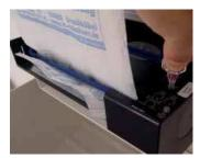
Press the button labelled "Manual operation" and the paper is automatically pulled in and dispensed from the device.
