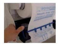
With the blue lever on the left side, raise the front paper guide with paper feed through.
