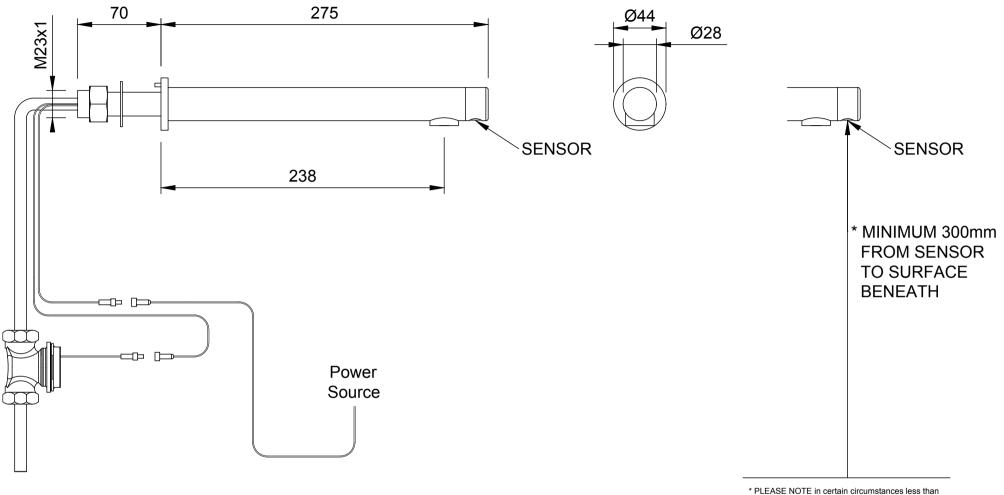
DOLPHIN SOLUTIONS LIMITED DOLPHIN PANEL MOUNTED INFRARED TAP - LONGER VERSION DBL1400 / DBL1425 PLEASE NOTE in certain circumstances less than 300mm is possible but we recommend a mock-up be created to test it in any specific situations to ensure less than 300mm does not cause any issues.
