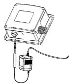
DC: put in  $4 \times AA$  alkaline batteries into the battery box
