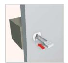
Push the integral disc along the toggle to make a snug purchase on the wall face. The toggle strands are rachetted to hold the disc in place.
