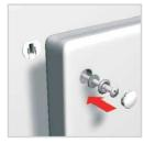
Align and engage the fixing bolt in the threaded toggle bar with washers engaged. The flat fender washer is to be inserted underneath the finishing washer. Finally, insert the snap-fit plastic covers in each fixing port.
