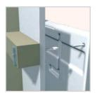
Cut off the surplus projection of the toggle and offer up the unit for fixing.
