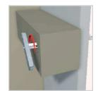
Twist toggle freely to gain purchase on the supporting member. There should be a minimum cavity clearance of 65mm to allow the toggle bar to turn.
